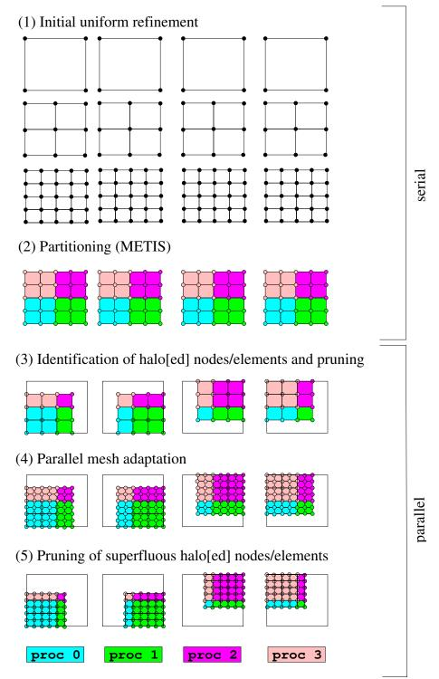
Figure 1.1 Sketch illustrating the phases of the parallel mesh adaptation procedure for a problem that is distributed over four processors. The columns illustrate the evolution of the mesh on each of the four processors. The colours of the objects indicate which processor is associated with them.
